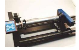
This photo shows a typical example of a larger part that requires a fixture plate on both the left and the right sides. Notice that the left side fixture plate is held in place with the 3-Jaw Chuck.
