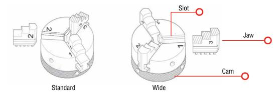
Pay particular attention to aligning the numbers as shown on the diagram when flipping the jaws! Failure to align the correct jaw in the correct slot will result in uneven spacing of the jaws when they are tightened.
