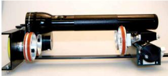
**Correct Setup:** The flashlight is horizontal to the X-beam
