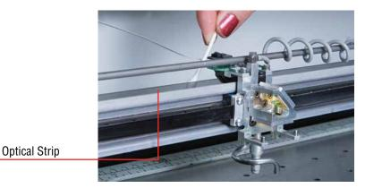
it is just a matter of removing the X-beam's protective cover and wiping off the optical encoder strip using a soft cotton cloth or cotton swab soaked in water or a mild dish washing soap.
