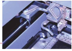
After cleaning the rails and bearings, clean off the table and the rest of the inside of the machine. Spending just a few minutes a week will pay off in the long run with better quality and performance.
