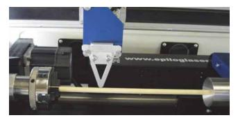
The 3-Jaw Chuck can be used with the standard 3" lens, or the optional 1.5" lens can be used to accommodate larger diameter pieces.
