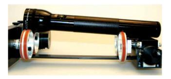
**Incorrect Setup:** The flashlight is not horizontal. Raise the right side of the flashlight by turning the jack screw.
