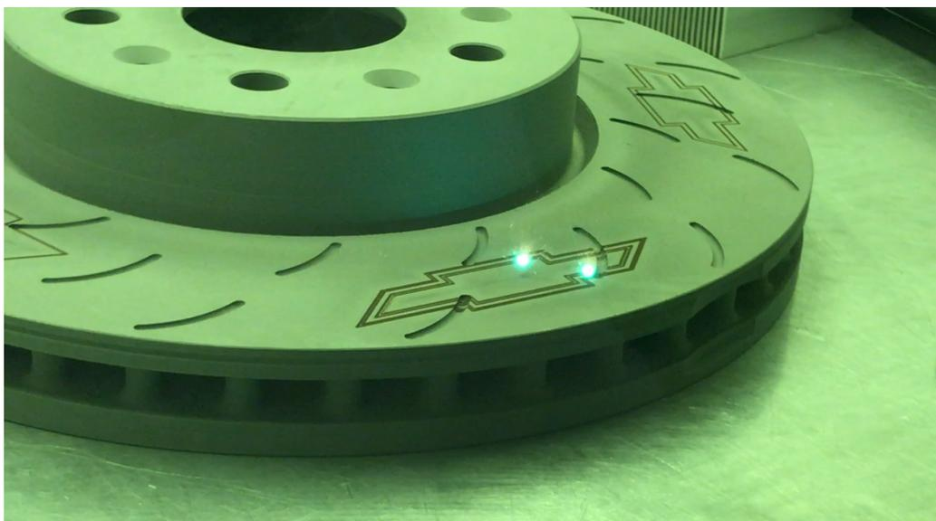
**Figure 1:** The G2 system engraving disc brakes. Source: Epilog Laser
