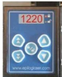
The display can show number is either inches or mm. The only indicator is if there is a decimal point showing on the display. A decimal indicates that the display is showing millimeters. To toggle between inches and millimeters, **press and hold the Lock/Unlock key** for several seconds until you see the display change. Once the display is set to the units you want, the Rotary Attachment will default to those units every time it is powered on.
