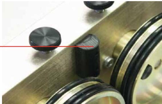
Use the scissor jack to raise the right side of the cylinder so that the engraving surface is horizontal. The photo below shows the same flashlight at a severe angle to horizontal. If your cylinder is not horizontal to the X-beam, the laser will lose focus as the carriage head moves across the flashlight. This causes the engraving quality on the right hand side to suffer dramatically.
