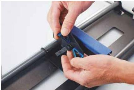
The splines on all the fixture plates can be reversed to accommodate parts using the inside diameter (ID) or outside diameter (OD). To reverse the spline orientation, pull the spring-loaded splines away from the plate and rotate them 180 degrees.
